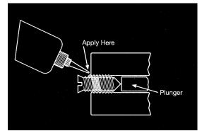
Avoid touching the bottle tip to the metal surface. Not recommended for pre-assembled threads in a blind hole.
