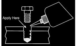
Assemble and tighten as usual. When tightening to established torque values, torque compensation is not required.
