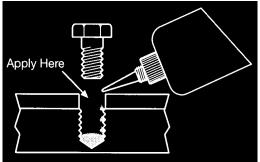
Assemble and tighten as usual. When tightening to 7. established torque values, torque compensation is not required.
