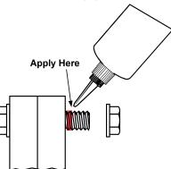
6. For Blind Holes, apply several drops down the female threads into the bottom of the hole. As threads are engaged, compressed air forces the product upwards into the threads.
